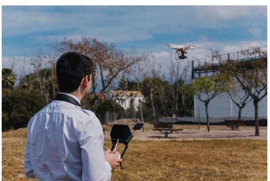
FIGURE 16 The drone pilot maintains a line of sight with the aircraft while piloting
