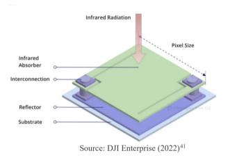
FIGURE 35 Diagram of a thermal sensor (microbolometer)
